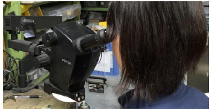
Fig. 2: Ryushi Takayama using a S8 APO (left) and one of his employees, Uchikoshi, using an A60 F (right) stereo microscope to inspect a surgical instrument component. Both microscopes from Leica Microsystems are used for inspection and quality control at TAKAYAMA Instrument.
